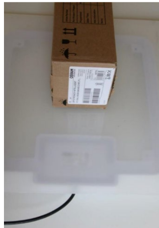
Figure 5: Orientation of the box to antenna ANT310/310
