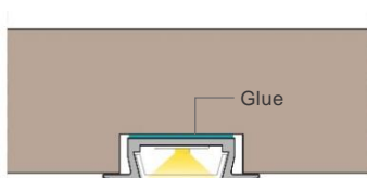
Recessed installation example with glue on wooden furniture
