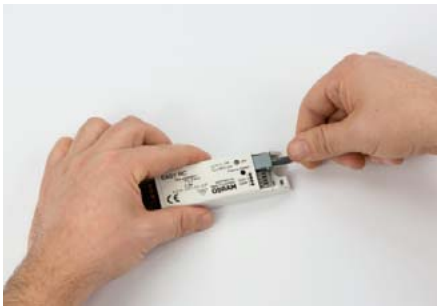
Installation of the radio receiver into the network behind the counter, connecting the cable to the OT EASY 80
