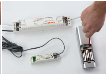
Teaching the wireless remote control using the push button
