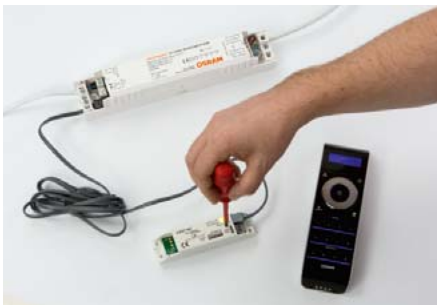
Teaching the wireless remote control using the push button
