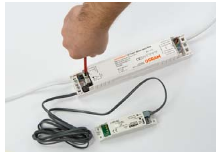
Connecting the mains power (at 230V~) to the OT EASY 80
