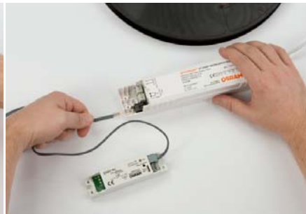
Installation of the radio receiver into the network behind the counter, connecting the cable to the OT EASY 80
