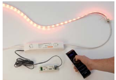
Commissioning the LED module using the push button (no PC etc. required)
