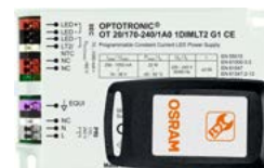
NFC scanner on LED driver
