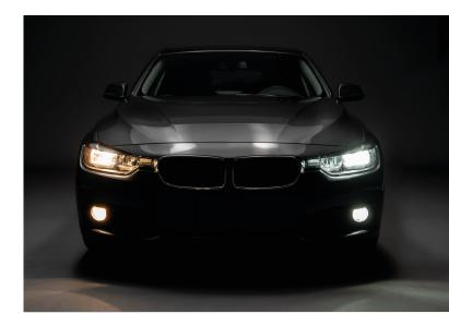
Making a difference: OSRAM LEDriving® FL lamps (right) do not only look cooler than conventional halogen lamps (left). They also provide more light.
