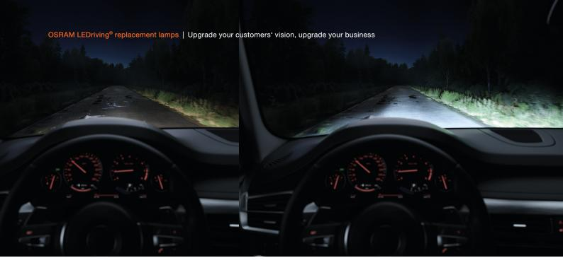
Daylight in the night: With a daylight-like colour temperature of 6,500 K, OSRAM LEDriving® HL and FL lamps (right) provide a higher contrast and thus improve visibility.
