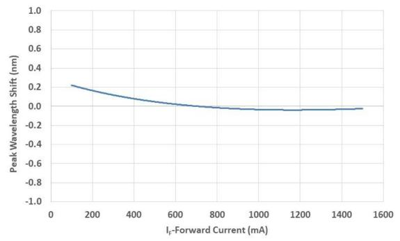
Figure 9: Typical peak wavelength shift vs. forward current @  $Tc = 25^{\circ}C$ .
