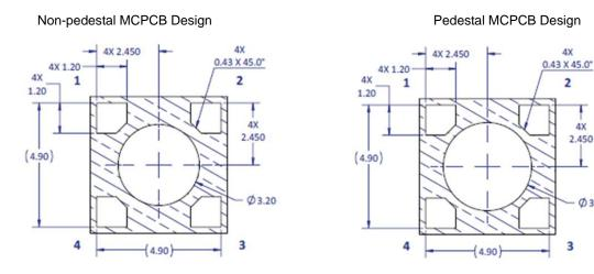
Figure 2b: Recommended solder mask opening for anode, cathode, and thermal pad for non-pedestal and pedestal design. Note for Figure 2b:
