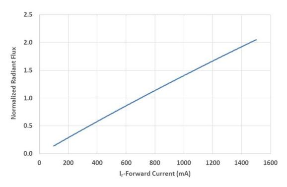
Figure 7: Typical normalized radiant flux vs. forward current @  $T_C = 25^{\circ}C$ .
