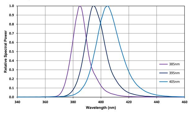
Figure 5: Typical relative spectral power vs. wavelength @  $T_C = 25^{\circ}C$ .
