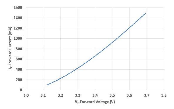
Figure 6: Typical forward current vs. forward voltage @  $T_c = 25^{\circ}C$ .
