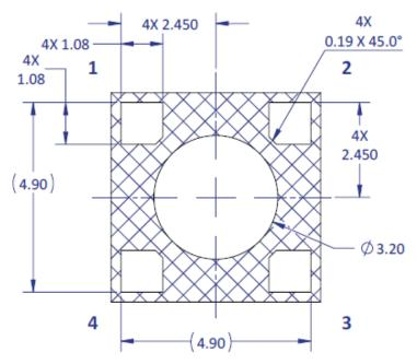
Figure 2c: Recommended solder mask opening for anode, cathode, and thermal pad for non-pedestal and pedestal design. Note for Figure 2c:
