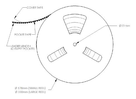
Figure 13: Emitter reel specifications (mm).
