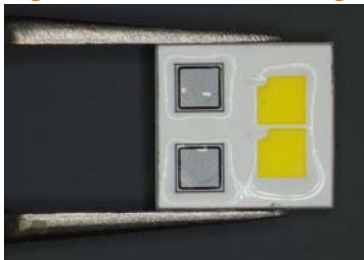
Figure 3: Manual Handling of the OSLON Submount CL
