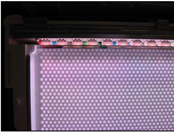
Figure 5: Upper left corner of the LED backlight in operation
