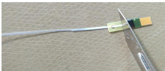
Figure 4: Cable Cutting Position
