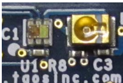
Figure 6. Single LDO recommended passive placement (shown on double sided PCB)
