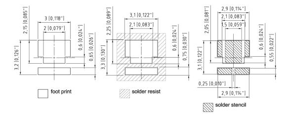
For superior solder joint connectivity results we recommend soldering under standard nitrogen atmosphere. Package not suitable for ultra sonic cleaning.
